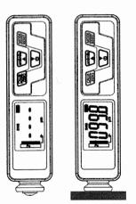
**"CON"**: the Continuous Measurement Mod Pressing "MODE" key to display CON, vertically ar directly placing the probe on the sample. The reading will continuously upgrade following with the prot moving, as showing below:
